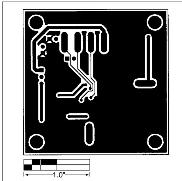
Figure 4. MAX1705 EV Kit PC Board Layout—Solder Side
