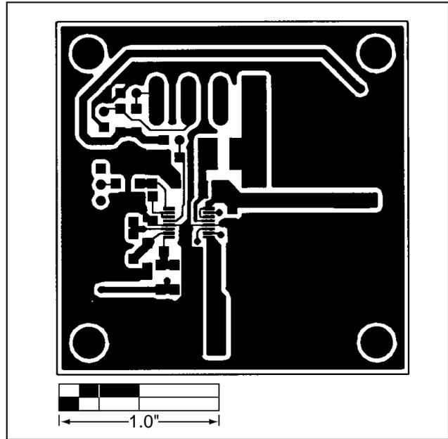
Figure 3. MAX1705 EV Kit PC Board Layout—Component Side
