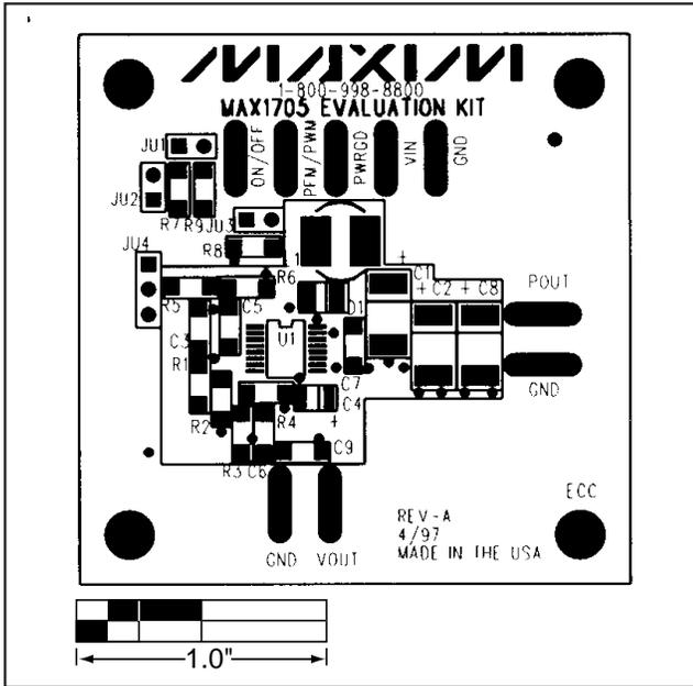
Figure 2. MAX1705 EV Kit Component Placement Guide—Component Side
